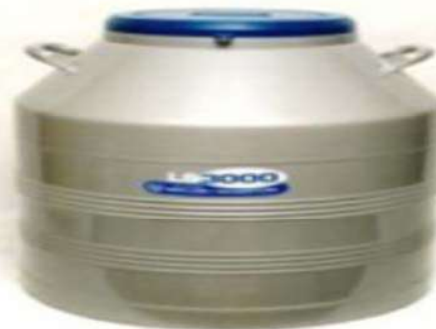
Figure 13. Liquid n 2 tank.
